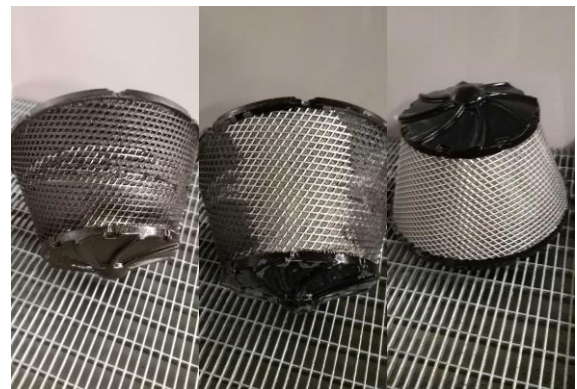
The example of a conical filter: Parts cleaning with low pressure hot cleaner – before and after in a minimal time span
