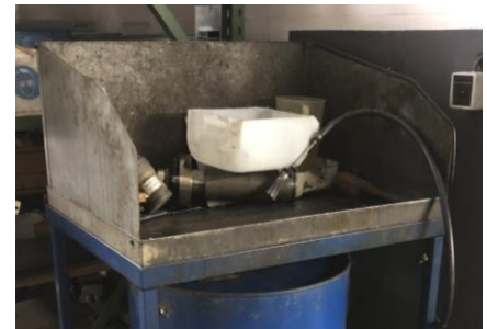
Washstands with brushes hit their limits with rough soilings and difficult geometries.
