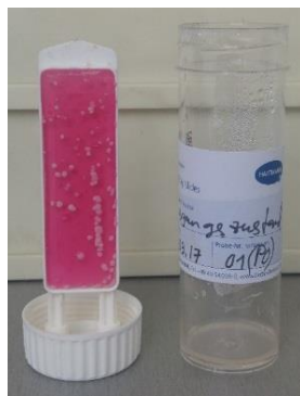
Coolant after three days: No thermal disinfection bacteria 10^4 cfu/ml fungi 10^4 cfu/ml (cfu = colony-forming units)
