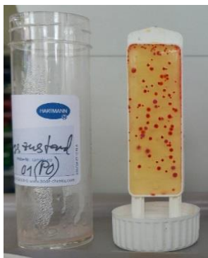
Coolant after three days: No thermal disinfection bacteria 10^4 cfu/ml fungi 10^4 cfu/ml (cfu = colony-forming units)
