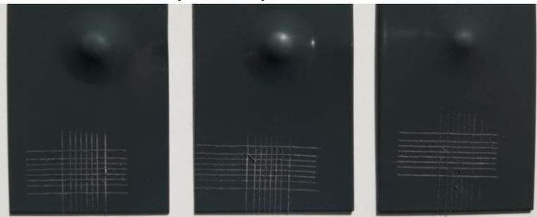
colours: Whenever two work pieces were submitted to Mr. Quality Control or to “the boss”, one degreased and powder coated using the traditional method and one using the method ph-cleantec, in no instance could they find a difference.
