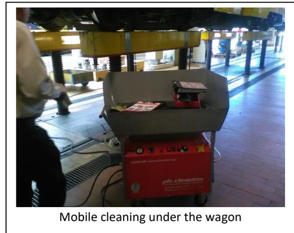
Another great advantage of low-pressure cleaning is that dirt remains in the unit resp. in the collector - there are no significant splash-back effects, dirt is neither carried through the factory floor by high pressure nor by solvents such as A-I cleaners. The employees do no longer stand in a cloud of droplets, and the protective clothing usually required for HP cleaners can be dispensed with. This makes cleaning much more comfortable and less cumbersome.
