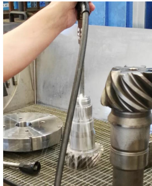
Internal cleaning of a deep blind hole in a shaft - detail
