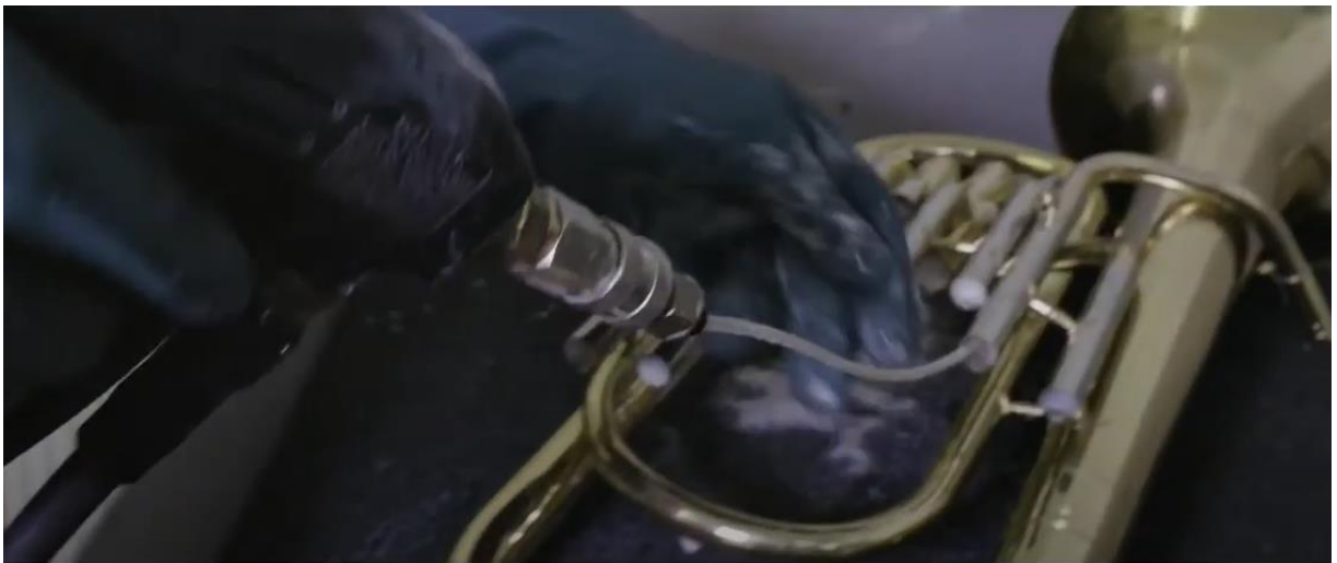
Cleaning the inside of a tube, example trumpet – here with flexible nozzle
