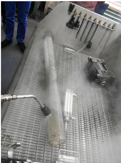
Cleaning the outside of a heavily contaminated glass tube – before
