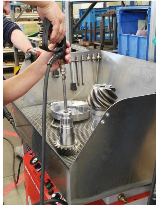
Cleaning the inside of a deep blind hole in a shaft
