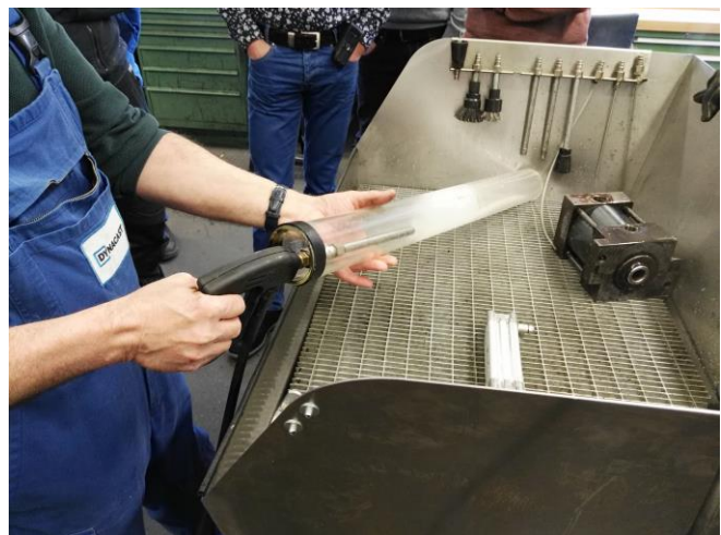
Cleaning the inside of the glass tube 1 minute later – finishing touches
