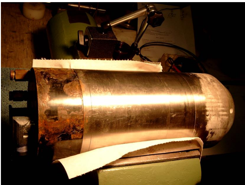
Machine tool spindle, uncleaned, courtesy UKF Universal-Kugellager-Fabrik, Berlin
