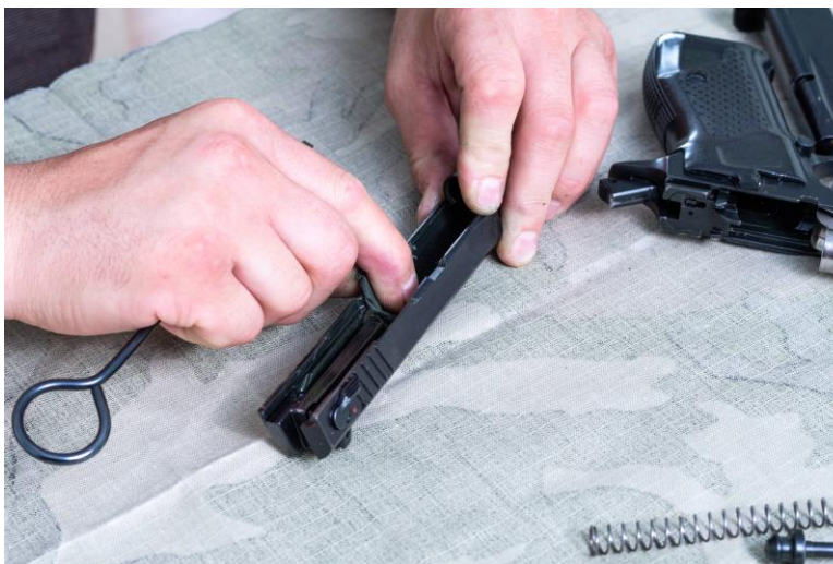
manual cleaning of a pistol – taken apart
