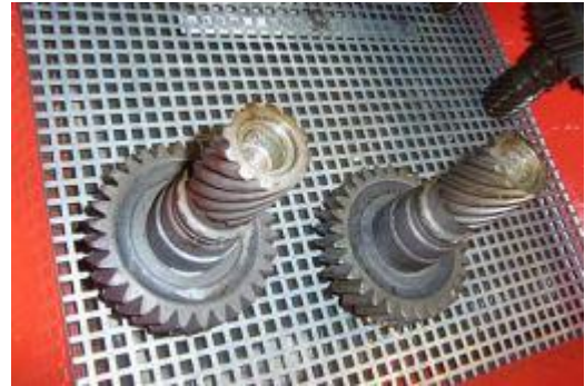
Retarder shafts with tempering oil
