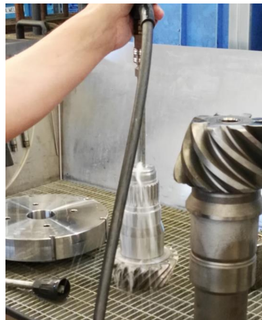
Manual internal cleaning of a blind hole in a retarder shaft - the process step can also be automated
