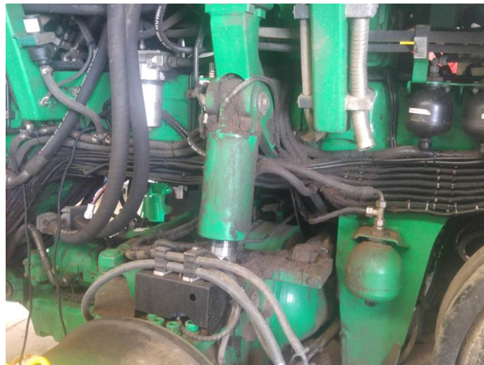
Hydraulic cylinder in the commercial vehicle sector - can be cleaned locally with low-pressure hot cleaning process
