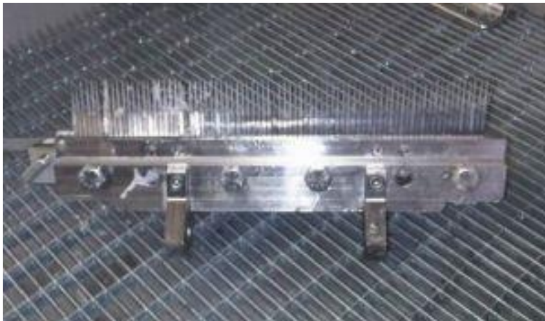
Glue comb, top left uncleaned with residue of dried adhesive
