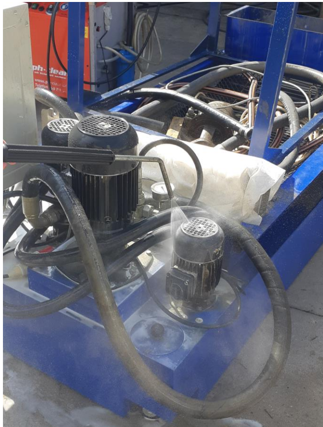
Cleaning electric motors for cooling lubricants: Cleaning is done with cooling lubricant when machine tool is in operation, or with water and low-dose alkaline cleaner.
