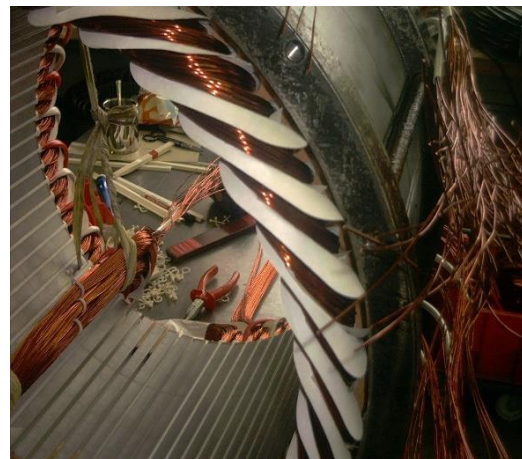
Electric motor: Stator coil
