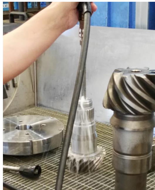
Cleaning the inside of a deep blind hole in a shaft - detail
