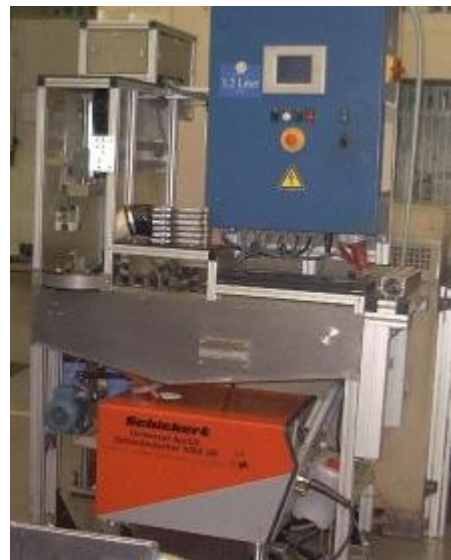
Simple parts cleaning system on the basis of low pressure hot cleaning technology
