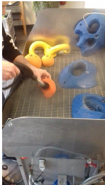
Cleaning of handholds and footholds in the parts cleaning level of a 1000 SR
