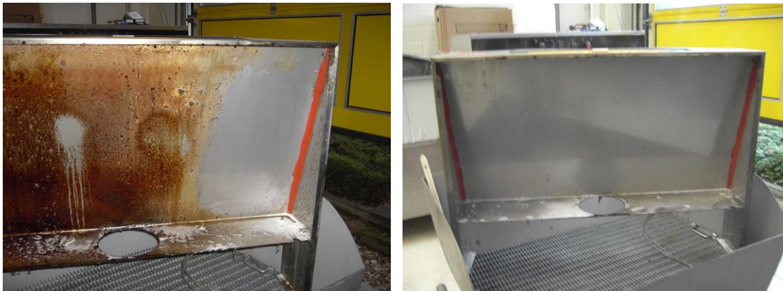
Fire damage cleaning - during and after cleaning in parts cleaning level of 1000 SR
