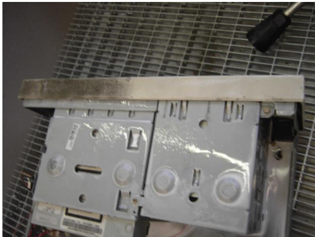
Gentle cleaning of hard disks with minor fire damage in parts cleaning level of 1000 SR
