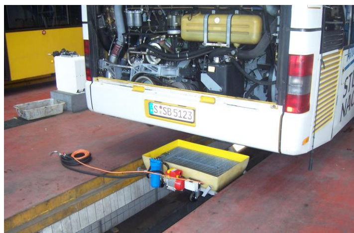
Use of the KW-FK collector in the pit. Frame size can be adapted to any pit thanks to extendable rods and rollers.
