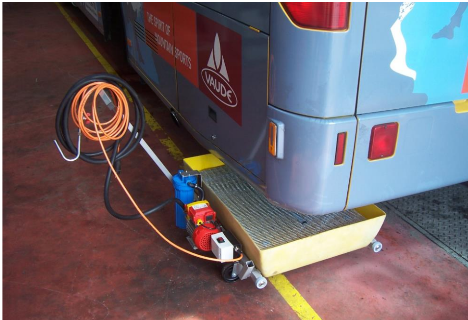
Coolant recycling collector 1000 KW-FK. The filter (blue), pump (red) and return hose (orange, with silver hook for hooking into the filler neck for the coolant) are clearly visible.
