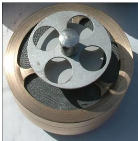
Soot filter after cleaning and polishing of the brass cage with polishing linen
