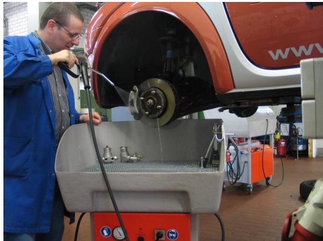
Car brake cleaning directly on the lifting platform saves dismantling and reassembly time, as well as travel time. Dirt water is collected in the unit and recycled.
