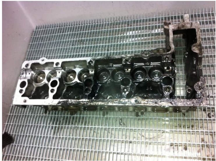
Parts cleaning, here the cylinder head of a Smart. Cleaned in a few seconds on the left, uncleaned on the right.
