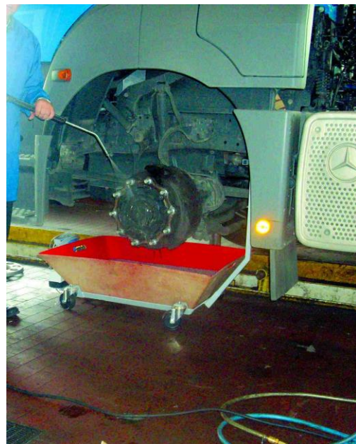
Brake cleaning at the pit – truck with dirt water collector
