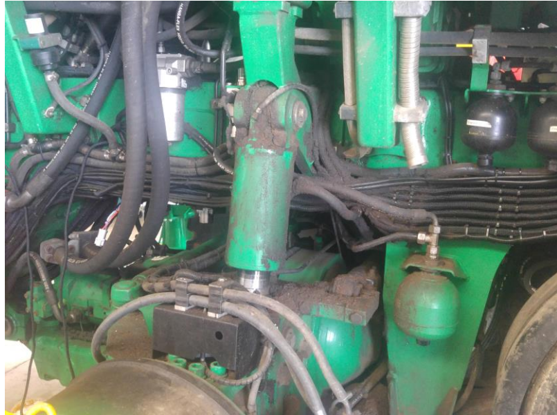
Cleaning of sensitive parts - here cable harnesses on a harvester - or of hydraulic parts is often possible without dismantling.
