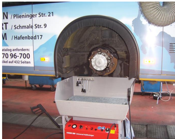
Brake cleaning directly at the lifting platform - Bus for public transport
